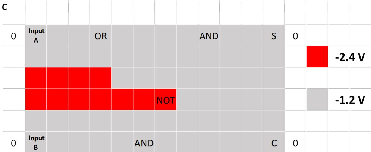
**Figure 2 | Logical circuit and plasmon mapping.** (a) Traditional half-adder logic circuit (AND, OR, NOT). (b) Upper Au gate mapping (inputs A and B at null). (c) Lower Au gate mapping for inverse plasmon generation (NOT logic).
