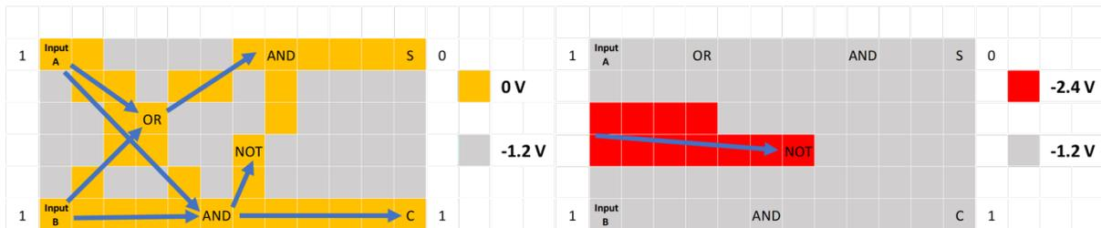
**Figure 3 | Half-adder plasmon processing.** (a): Input A=1, B=0. (b): Input A=0, B=1. (c): Input A=1, B=1. Outputs are derived from plasmon annihilation/transmission.
