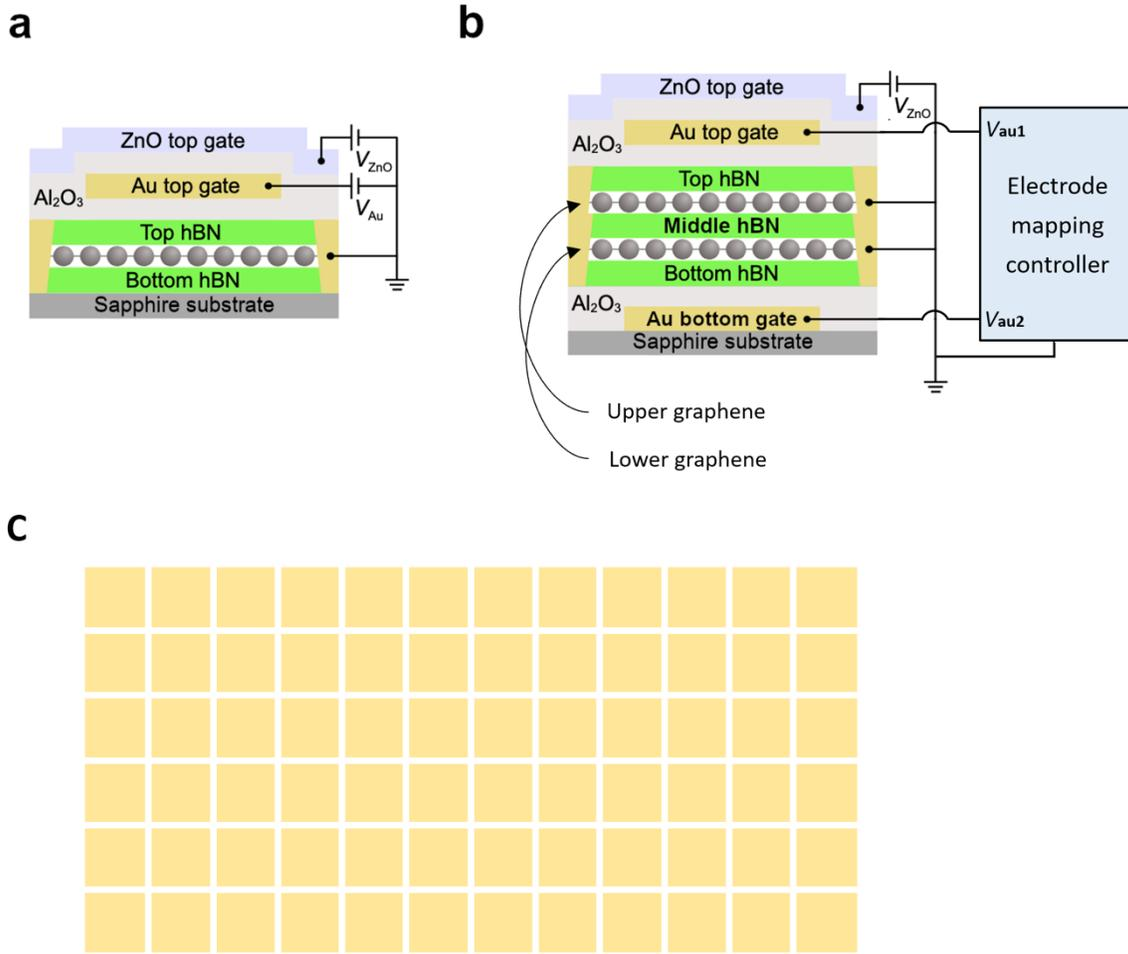
**Figure 1 | Cross-sectional view of the half-adder chip.** (a) Original design from Ref. (1). (b) Modified design with an additional graphene layer and Au bottom gate. (c) Overhead view of the latticed Au gates, controlled individually by the electrode mapping controller.
